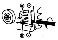
Feed the chain around the chain sprocket into the bar groove (Fig. 35). Cutters (the sharp edge on top) must point forward toward bar nose. Insure the chain drive links engage the chain sprocket and the sprocket nose on the bar.
