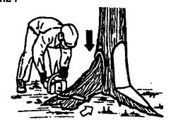
When felling, assume a balanced body position (Fig. 8). Position the feet parallel and apart to obtain a steady stance and stand at the side of the tree. Lower the point of gravity by bending the knees (comfortably arch your back). Keep the saw near the body, hold it firmly with both hands, and lock the thumbs under the handlebar at all times.
