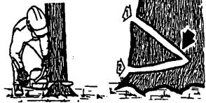
The exception is when the tree is on a slope; then the lower cut should be on an upward angle to cut a larger, more open wedge and to gain greater control during the fall of the tree (Fig. 11).
