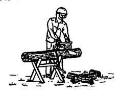
Free hanging ends can be cut off without risk of bar pinching. But if the wood is not to split or tear, make an undercut (underbucking, Fig. 20, 1) of about 1/3 the depth of the log diameter, then apply the finishing cut (overbucking, Fig. 20, 2).
