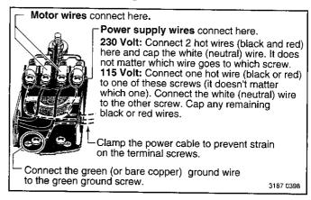
Figure 17 - Pressure Switch Wiring
