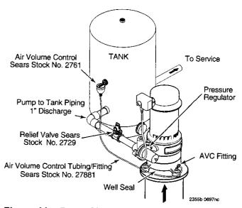
Figure 11 - Pump With Standard Tank
