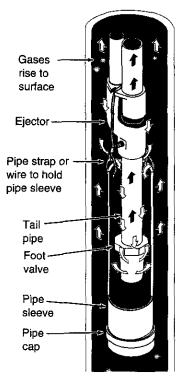
Figure 20 - Gas/Air Control in Well
