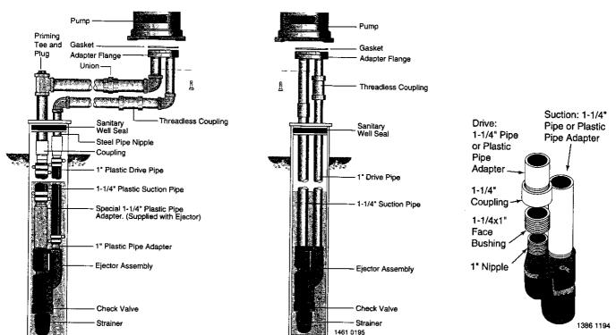
Figure 6 – Offset Installation Plastic Pipe Shown
