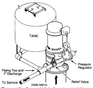
Figure 12 – Pump With Captive-Air® Tank
