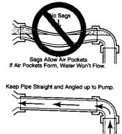
Figure 3 - No Air Pockets in Suction Pipe
