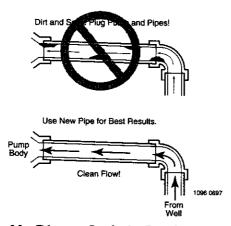
Figure I - No Dirt or Scale in Suction Pipe
