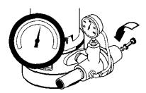
Figure 19C - Close Regulator Valve until Pressure Stabilizes
