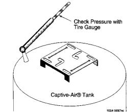
Figure 13 - Checking Tank Pre-charge
