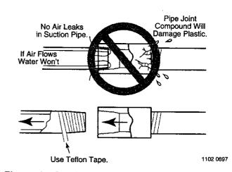
Figure 4 - Suction Pipe Must Not Leak
