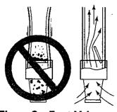
Figure 2 – Foot Valve Must Work Freely
