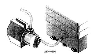
Figure 2B – Connect pump to spigot for use with sprinklers. Connect with adapters supplied with pump.
