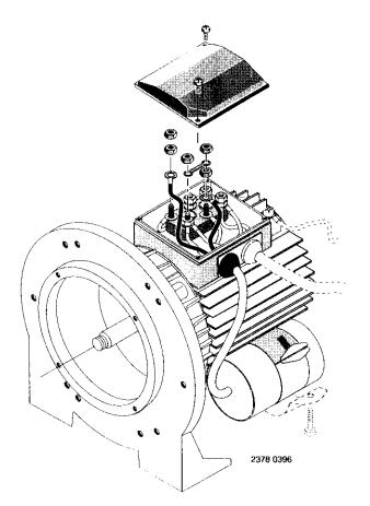
Figure 5 – Capacitor replacement. Unplug pump before doing any work on it. Discharge capacitor by shorting capacitor lead wires together before removing it.
