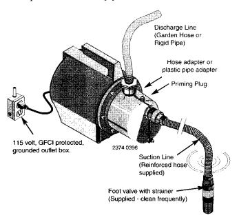
Figure 1 - Typical Installation
