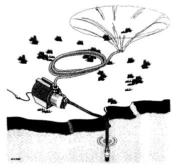
Figure 4 – Sprinkler pumping from pond. Pump can supply one to three sprinklers depending on conditions.
