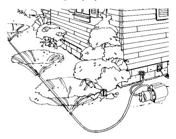
Figure 3 – Typical sprinkler application. Pump can supply up to three sprinklers.
