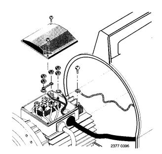
Figure 6 – Shroud replacement. Unplug pump before doing any work on it. Be sure that green ground wire is solidly connected to grounding terminal (marked (\*\*)) before reinstalling shroud. See Steps I and IO, Page 6, for shroud fastenings.
