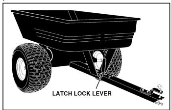
**LATCH LOCK LEVER** Locks the front of the cart to the tongue and releases it for dumping.
