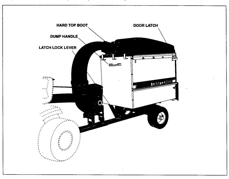
HARD TOP BOOT Connects the plastic elbow to the hard top, directing discharged material into the cart.
