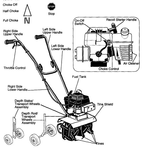
Throttle Control – Controls the engine speed and the tine rotation. This cultivator is equipped with a centrifugal clutch that engages the tine drive system when the engine speed is increased.
