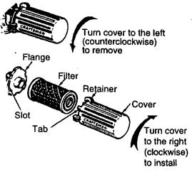
**CAUTION:** Never run the engine without the air cleaner element installed. A defective air cleaner can result in loss of engine power and can cause excessive wear or damage to the engine components if dirt or dust is permitted to enter the engine through the carburetor. A damaged air cleaner, or one that is clogged with dust or dirt should be replaced immediately.
