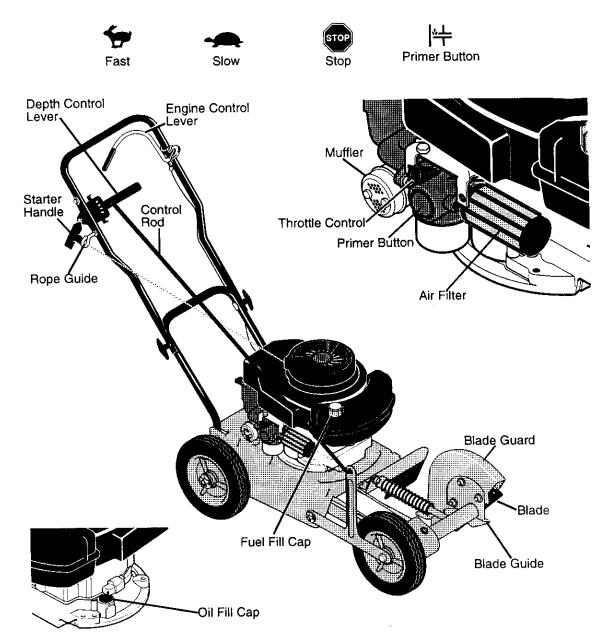
Throttle Control – Used to control the engine speed.
