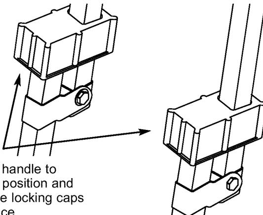
Lift the handle to upright position and slide the locking caps into place
