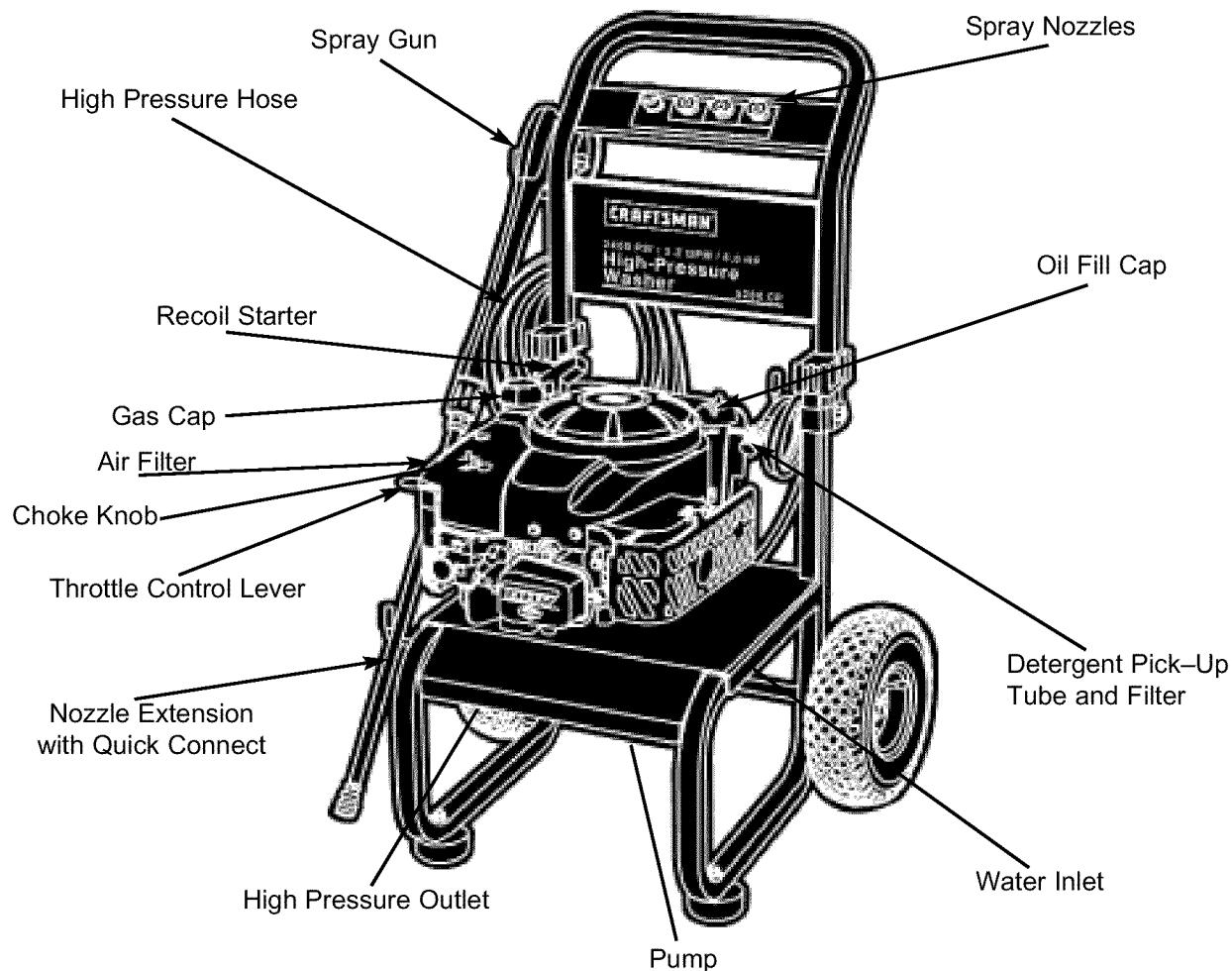
**Air Filter** – Dry type filter element limits the amount of dirt and dust that gets in the engine.
