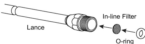
4. Place the o-ring into the recess. Push the o-ring snugly against the in-line filter screen.
