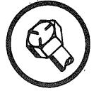
A GRADE 5 HEAT TREATED BOLT CAN BE IDENTIFIED BY THREE LINES ON THE BOLT HEAD AS SHOWN AT LEFT.
