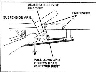
FRONT-TO-BACK ADJUSTMENT (See Figs. 22 and 23) -IMPORTANT: DECK MUST BE LEVEL SIDE-TO-SIDE. IF THE FOLLOWING FRONT-TO-BACK ADJUSTMENT IS NECESSARY, BE SURE TO ADJUST BOTH FRONT LINKS EQUALLY SO MOWER WILL STAY LEVEL SIDE-TO-SIDE.
