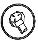
A GRADE 5 HEAT TREATED BOLT CAN BE IDENTIFIED BY THREE LINES ON THE BOLT HEAD AS SHOWN AT LEFT.
