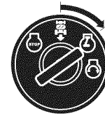
Engine "On" Position (Normal Operating)
