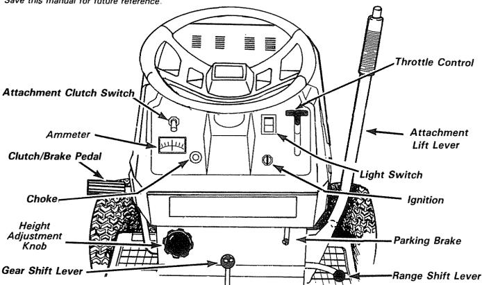
**ATTACHMENT CLUTCH SWITCH:** Pull switch out and up to engage attachment. There will be an engine hesitation as the clutch engages.
