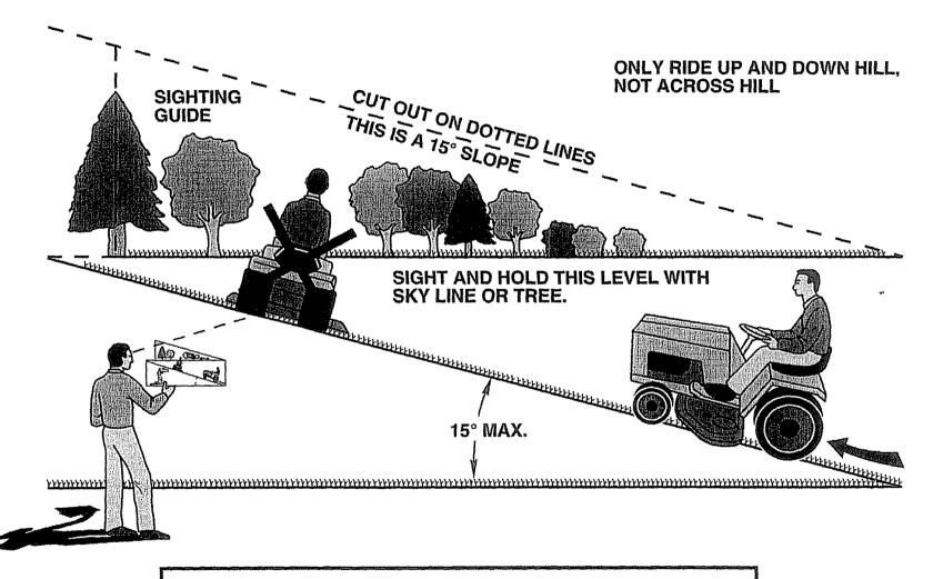
Operate your Tractor up and down the face of slopes (not greater than 15°), never across the face. Make turns gradually to prevent tipping or loss of control. Exercise extreme caution when changing direction on slopes.
