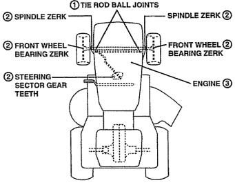
(1) SPRAY SILICONE LUBRICANT (MOVE BOOTS TO LUBRICATE)
