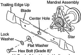
\*A Grade 8 heat treated bolt can be identified by six lines on the bolt head.
