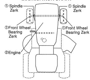
①General Purpose Grease ②Refer to Maintenance "Engine" Section
