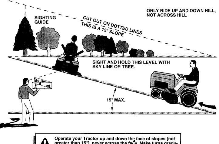
Operate your Tractor up and down the face of slopes (not greater than 15°), never across the face. Make turns gradually to prevent tipping or loss of control. Exercise extreme caution when changing direction on slopes.
