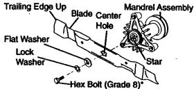
\*A Grade 8 heat treated bolt can be identified by six lines on the bolt head.
