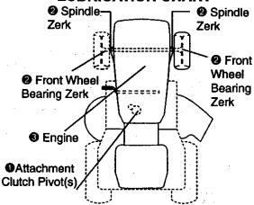
SAE 30 or 10w30 Motor OIL General Purpose Grease Refer to Maintenance "Engine" Section
