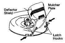
ACAUTION: Do not remove deflector shield from mower. Raise and hold shield when attaching mulcher plate and allow it to rest on plate while in operation.
