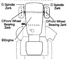
**®SAE 30 or 10w30 MOTOR OIL** @Refer TO Maintenance "ENGINE" Section IMPORTANT: Do not oil or grease the pivot points which have special nylon bearings. Viscous lubricants will attract dust and dirt that will shorten the life of the self-lubricating bearings. If you feel they must be lubricated, use only a dry, powdered graphite type lubricant
