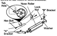
**INSTALL MOWER AND DRIVE BELT** Be sure tractor is on level surface and mower suspension arms are raised with attachment lift control. Engage parking brake.
