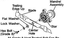
\*A Grade 8 Heat Treated Bolt Can Be Identified By Six Lines On The Bolt Head
