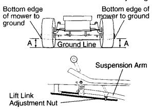
FRONT-TO-BACK ADJUSTMENT IMPORTANT: Deck must be level side-to side. If the following front-to-back adjustment is necessary, be sure to adjust both front links equally so mower will stay level side-to-side.
