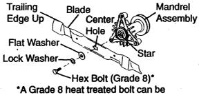
identified by six lines on the bolt head.
