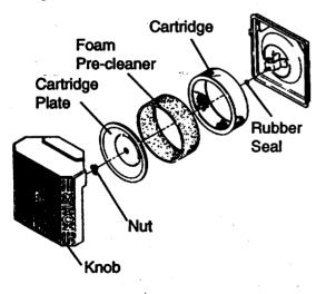
**NOTE:** Do not wash the paper cartridge or use pressurized air, as this will damage the cartridge.
