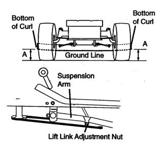
FRONT-TO-BACK ADJUSTMENT IMPORTANT: Deck must be level side-toside. If the following front-to-back adjustment is necessary, be sure to adjust both front links equally so mower will stay level side-to-side.
