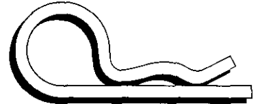
(3) Retainer Springs (double loop)
