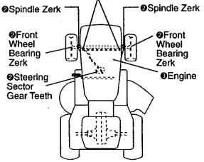
OSpray Silicone lubriant (Move Boots to Lubricate) **O**General Purpose Grease ØRefer to Maintenance "ENGINE" Section
