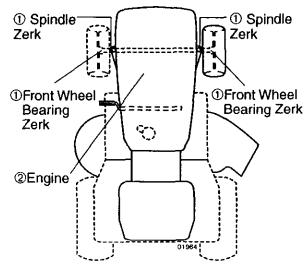
General Purpose Grease ② REFER TO Maintenance "ENGINE" SECTION
