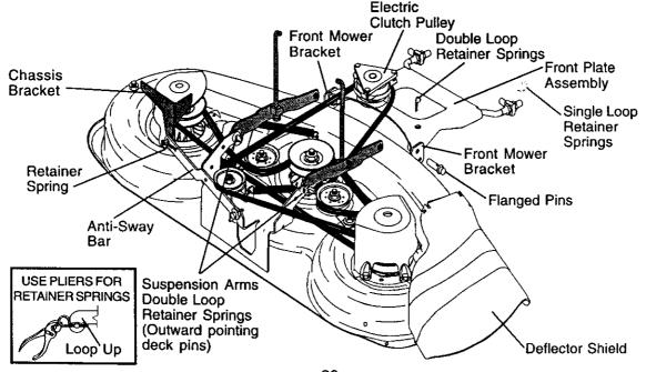
Position front plate assembly between front mower brackets. Raise deck and plate assembly to align holes and insert flanged pins. Secure pins with double loop retainer springs between the plate and mower brackets.
