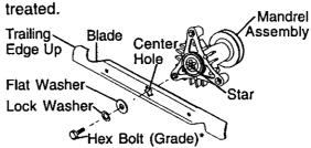
\*A Grade 8 heat treated bolt can be identified by six lines on the bolt head.
