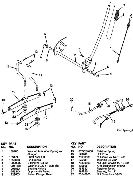
Arm Suspension Mower Retainer Spring Bearing, Pvt. Lift 139868
