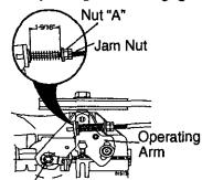
Do not touch this nut. If further brake adjustment is necessary contact a Sears or other qualified service center.
