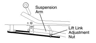
FRONT-TO-BACK ADJUSTMENT IMPORTANT: Deck must be level sideto-side. If the following front-to-back adjustment is necessary, be sure to adjust both front links equally so mower will stay level side-to-side.
