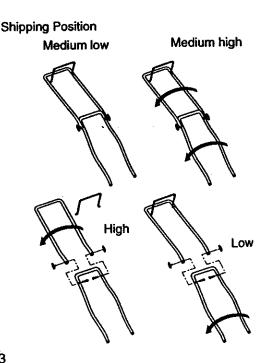
**ACAUTION:** The operator presence control bar must pivot freely to permit blade/ brake engagement when control bar is released. Do not overtighten the fasteners holding the controls to the upper handle.
