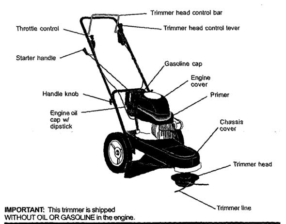
Trimmer head control bar - must be held down to the handle to engage trimmer head. Release to stop the trimmer head. Primer - pumps additional fuel from the carburetor to the cylinder for use when starting a cold engine.
