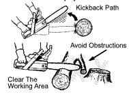
▲ WARNING: Avoid kickback which can result in serious injury. Kickback is the backward, upward or sudden forward motion of the guide bar occurring when the saw chain near the upper tip of the guide bar contacts any object such as a log or branch, or when the wood closes in and pinches the saw chain in the cut. Contacting a foreign object in the wood can also result in loss of chain saw control.
