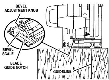
ALIGN INNER BLADE GUIDE NOTCH ON SAW BASE WITH LINE OF CUT AS SHOWN WHEN MAKING 45° BEVEL CUTS
