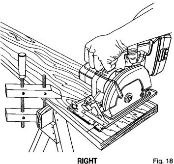
Depress the lock-off button and squeeze the switch trigger to start your saw. **Always** let the blade reach full speed, then guide your saw into the workpiece.
