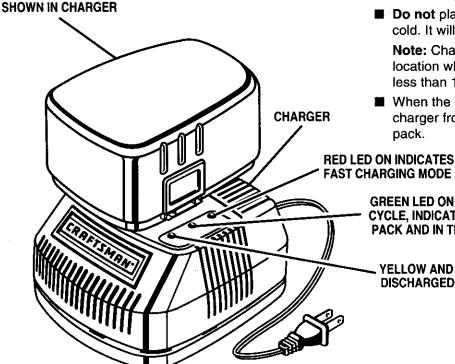
GREEN LED ON AFTER FAST CHARGING CYCLE, INDICATES FULLY CHARGED BATTERY PACK AND IN TRICKLE CHARGE MODE.
