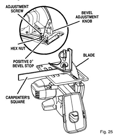
Your saw has a positive 0° bevet stop, that has been factory adjusted to assure 0° angle of your saw blade when making 90° cuts. However, misalignment can occur during shipping.
