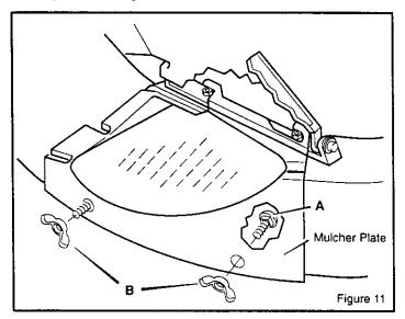
2. Slide the **mulcher plate** toward the front (Figure 12). Make sure the **tabs** on the **mulcher plate** are not locked behind the **nuts**.
