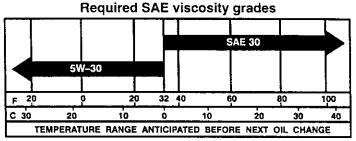
NOTE: Although multi-viscosity oils (5W30, 10W30, etc.) improve starting in cold weather, these multi-viscosity oils will result in increased oil consumption when used above 32<sup>0</sup> F. Check the engine oil level more frequently to avoid possible engine damage from running low on oil.
