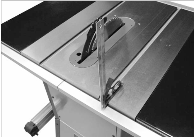
Figure 26 - Check parallelism of rails to table with combination square. Check at several locations along rail.
