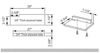
Attach auxiliary fence to rip fence with two "C" clamps. (Fig. JJ)
