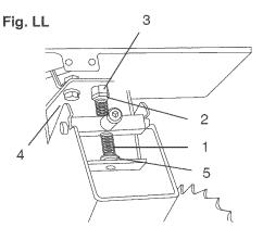
Place a small amount of dry lubricant on height regulating bolt (1). This must be kept clean and free of sawdust, gum, pitch, and other contaminants for smooth operation.
