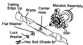
\*A Grade 8 heat reated bolt can be identified by six lines on the bolt head.
