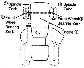
① SAE 30 OR 10W30 MOTOR OIL② Refer to Maintenance "ENGINE" Section
