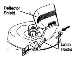
ACAUTION: Do not remove discharge guard from mower. Raise and hold guard when attaching mulcher plate and allow it to rest on plate while in operation.
