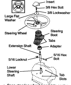
Snap steering wheel insert into center of steering wheel.
