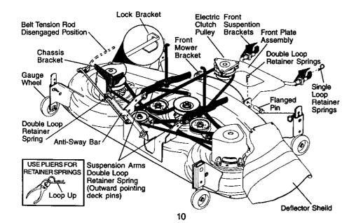
NOTE: To assist in locating hole in flanged pin, the hole in pin is inline with notch on head of pin. If necessary, move mower side-to-side to give space between plate and mower brackets. IMPORTANT: Check belt for proper routing in all mower pulley grooves.
