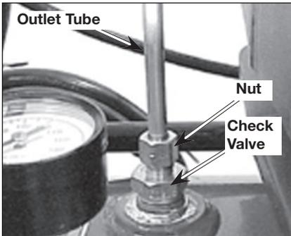
6. Apply sealant to the check valve threads. Reinstall the check valve (turn clockwise).
