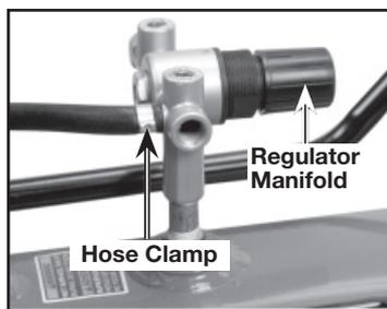
6. Apply pipe sealant to new regulator manifold and assemble, tighten with wrench.
