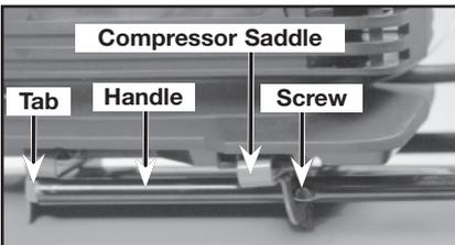
**CAUTION** It will be necessary to brace or support one side of the outfit when installing the wheels because the compressor will have a tendency to tip over.
