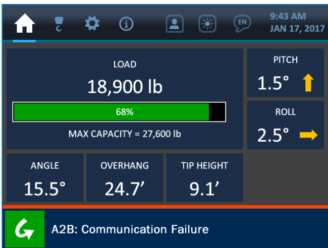
Showing Component Communication Error
