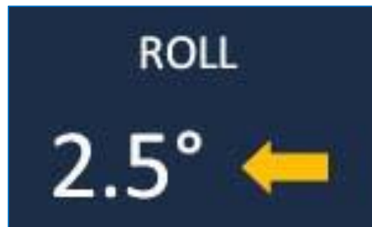
'Inverted' orientation of Roll parameter, showing a roll to the right side of 2.5^\circ
