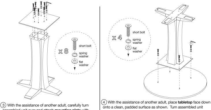
assembled unit over and attach **mounting plate** with 8**short bolts**, 8 **spring washers** and 8 **flat washers** using an allen wrench as shown.
