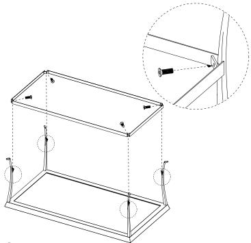
2 Fit **shelf** into position, aligning holes in shelf corners with holes on legs. Secure with 1 **allen head bolt** per leg and fully tighten each with **allen wrench**.
