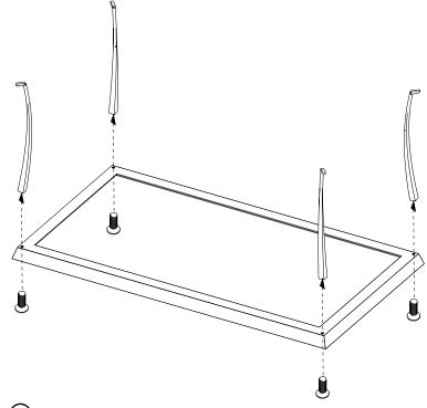
1) Place **top frame** upside down. Loosely attach each **leg** by inserting 1 **allen head bolt** through the top frame and into the corresponding hole in the top of each leg. Do not fully tighten.
