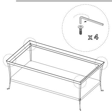
4 With the assistance of another adult, place table assembly in an upright position. Fully tighten all 4 allen head bolts in top frame with the allen wrench.
