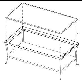
5 Remove the adhesive backer from 4 **rubber bumpers** and place over each exposed bolt head in the top frame. Fit **glass top** into position. Assembly is now complete.
