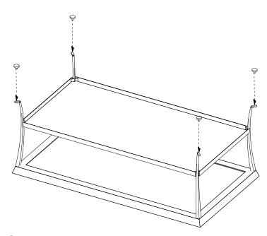
3 Insert 1 **leveller** into threaded hole on the bottom of each leg.
