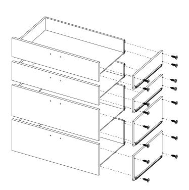
11) Fit the remaining small and large drawer side panels into position, securing with 4 short wood screws per panel.
