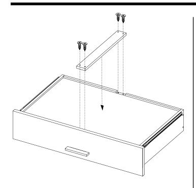
13) Turn all the drawers upside down. Attach 1 drawer support to the bottom of each drawer with 4 short wood screws. Repeat for the remaining 3 drawers.
