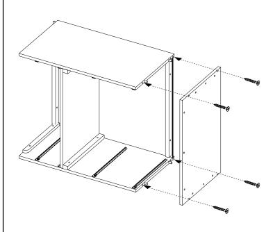
4 Fit **bottom panel** onto dowels in side panels and bottom of back panel. Secure with 4 **long wood screws**.
