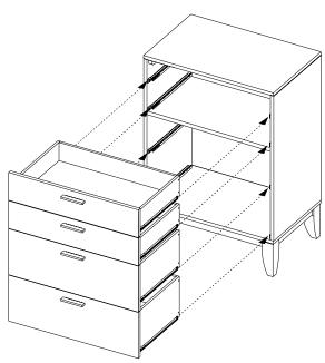
(14) Insert drawers into the case, fitting wheels on drawer assemblies into the metal tracks of the case drawer slides. Assembly is now complete.
