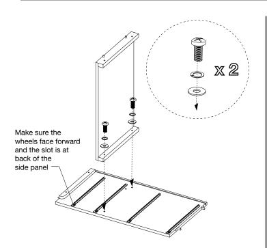
1 Attach middle panel to left side panel with 2 short machine screws, 2 spring washers and 2 small flat washers. Tighten with a phillips head screwdriver.
