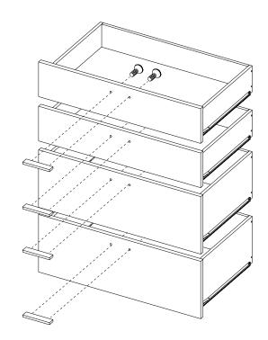
(12) Attach metal pulls to the **small** and **large drawer faces** using 2 **oval head screws** per drawer.
