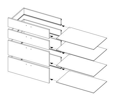
① Slide 4 **drawer bottoms** into the slots at the base of the drawer side, front and back panels.
