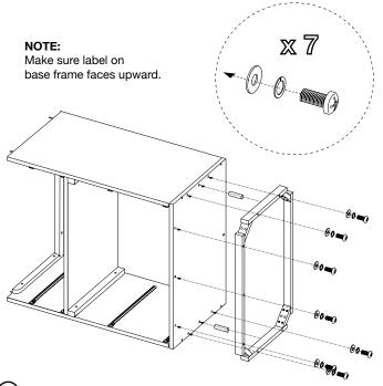
Insert 2 wood dowels into top of base frame.
