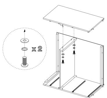
3 Fit dowels of middle panel and back panel into corresponding holes and slot in right **side panel**. Secure with 2 **short machine screws**, 2 **split washers** and 2 **small washers**.
