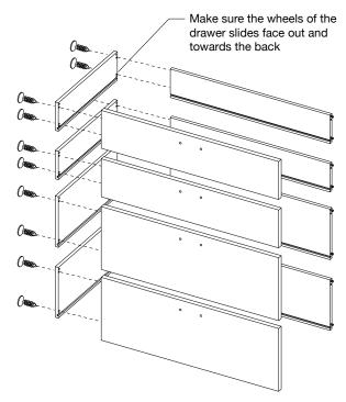
9 Using 4 **short wood screws** per panel, attach the **small** and **large drawer sides** to the **small** and **large front** and **backs**.
