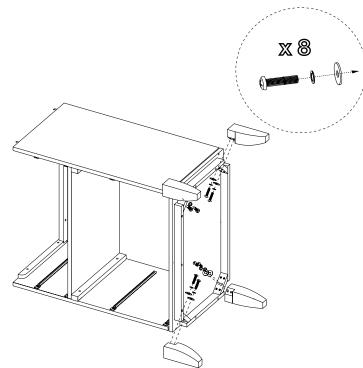
6 Secure 4 legs to base frame with 8 long machine screws, 8 spring washers and 8 large flat washers.
