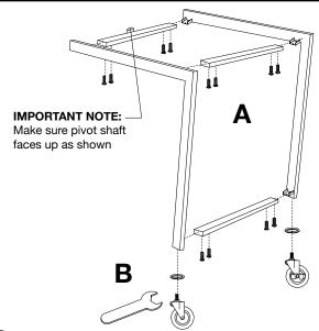
3 A. Fit 2 return crossbars and 1 pivot crossbar onto corresponding brackets on the right and left return frames as shown. Secure with 4 short bolts per crossbar, fully tightening each with the allen wrench.
