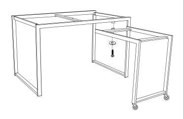
4 With the assistance of another adult, fit return assembly underneath desk assembly, aligning hole in pivot crossbar with hole in underside of front frame. Attach with 1 long bolt and 1 flat washer, securing with the allen wrench.
