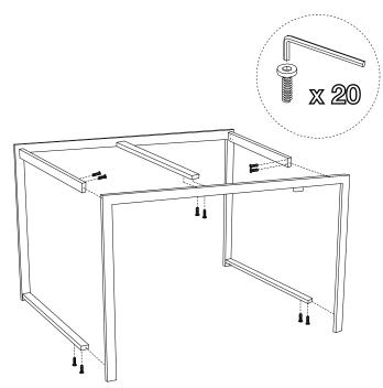
2 Fit brackets of **front frame** into ends of crossbars. Secure each crossbar with 2 **bolts**, fully tightening with the **allen wrench**. At this point, fully tighten 10 bolts installed in Step 1 with the allen wrench.
