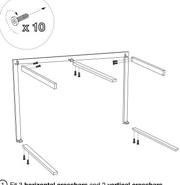
(1) Fit 3 horizontal crossbars and 2 vertical crossbars onto the brackets as shown. Loosely attach each crossbar with 2 small bolts. Do not fully tighten the bolts.
