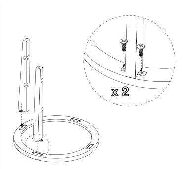
1) Place **top** face down on a padded surface. Position 2 **legs** as shown, fitting metal brackets into corresponding holes. Loosely attach with 2 **short bolts** per leg. Do not fully tighten the bolts.
