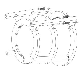
3 Attach remaining 2 **legs** as shown, fitting leg slots into corresponding slots in shelves. Loosely attach each leg to top with 2 **short bolts**. Do not fully tighten the bolts.
