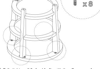
(5) Fully tighten all 8 **short bolts** with the **allen wrench**. With the assistance of another adult, lift assembled unit into an upright position. Assembly is now complete.
