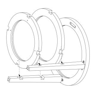
2 Turn top assembly on its side. Fit slots of **middle shelf** and bottom shelf into corresponding slots on legs as shown.
