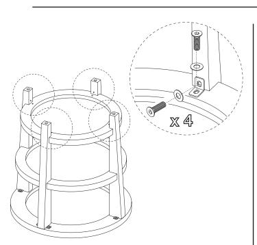
4) With the assistance of another adult, turn table assembly upside down. Attach 1 **bracket** at each leg and bottom shelf intersection. Secure each with 2 **long bolts** and 2 **washers**. Fully tighten with the **allen wrench**.
