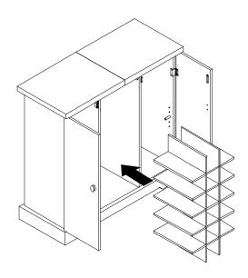
7 Fit assembled bottle grid into cabinet assembly as shown.
