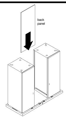
2 With assistance of another adult, carefully turn over unit. Insert **back panel** into corresponding grooves of each cabinet as shown.
